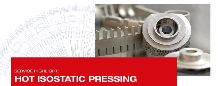
Hot isostatic pressing (HIP) improves the mechanical properties of cast or additive manufactured parts by bringing them to very high temperatures in a sealed chamber capable of generating very high pressures. It's becoming a preferred thermal process for aerospace parts that are 3D printed using selective laser or electron beam sintering technology.
